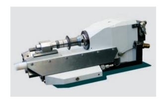
Universal-Shifting hobbead for hobbing of gears and for milling of single and multi start worms with a maximum hob length of 110 mm and 70 mm shifting.
